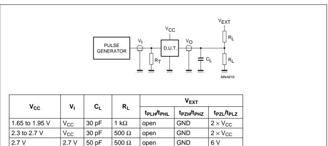
R<sub>L</sub> = Load resistor.
